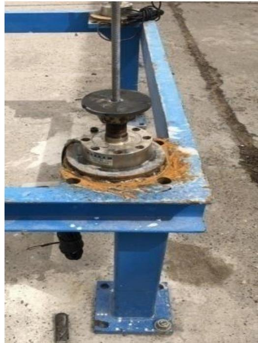
**Fig. 5. Fix load cell on stand and bolted stand with earth.**
