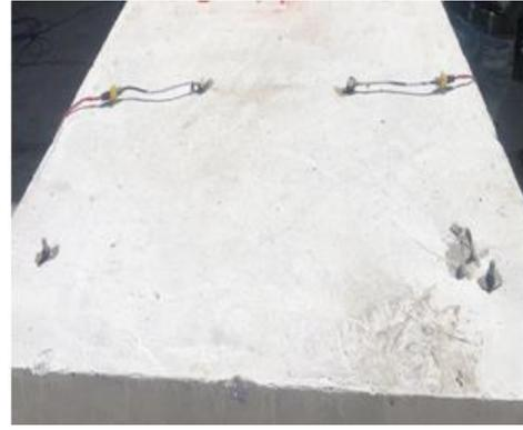
Fig. 7. Accelerometer on the surface of specimen.
